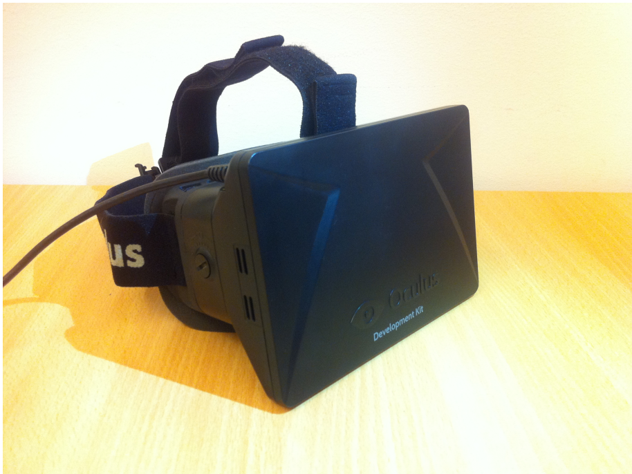
Figure 3.9: The Oculus Rift, the HMD used during the development of Breach.
